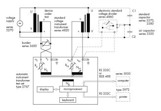
**3. Current and voltage transformer measurement part** Measurement ranges for
