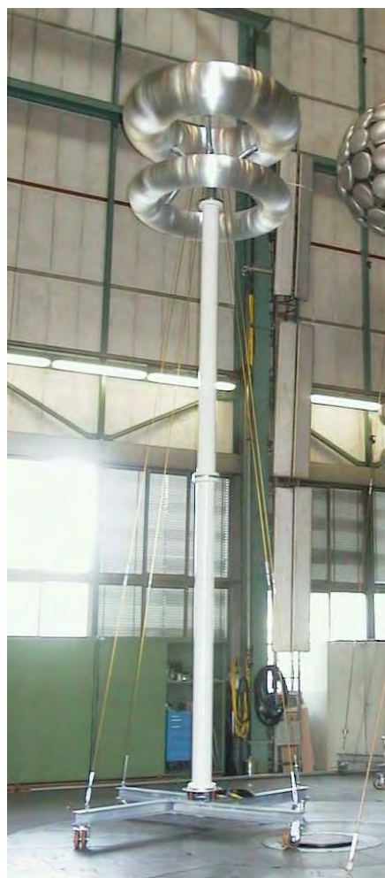
2400 kV impulse voltage divider
