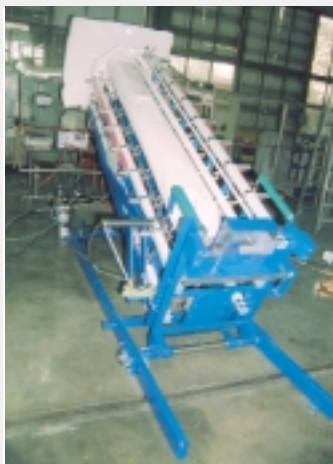
Mobile on-site impulse voltage test system for charging voltages of 800 kV. The automatic hydraulic erection system allows a very fast assembling and disassembling. Suitable for testing large Power Transformers.
