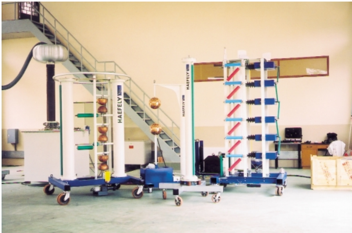
Impulse Voltage Test System SGSA, 600 kV, 30 kJ including MAFS and KFS
