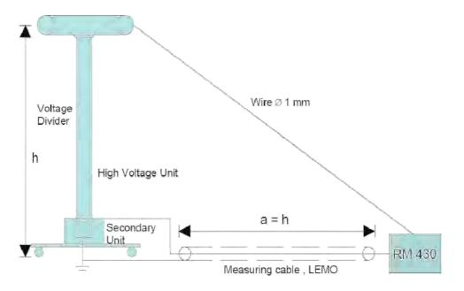
To measure a voltage divider the ratio meter RM430 is connected as shown above
