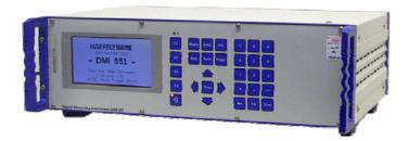
The Digital Measuring Instrument DMI 551 is a microprocessor controlled device for measuring AC, DC and impulse voltages. The instrument can also be used for firing a generator or a chopping sphere gap and to trigger an oscilloscope or any other measuring device. The triggers can be set for delays in time and in phase.
