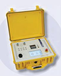
The **5478 portable teraohmmeter** is a multipurpose digital tester intended for analyzing, inspecting and maintaining any high voltage insulations.
